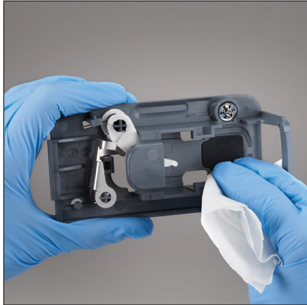
4. Clean the entire base using a lint-free wipe or cotton swab dampened with 70% isopropyl alcohol, mild liquid soap and water, or a 10% bleach solution.
